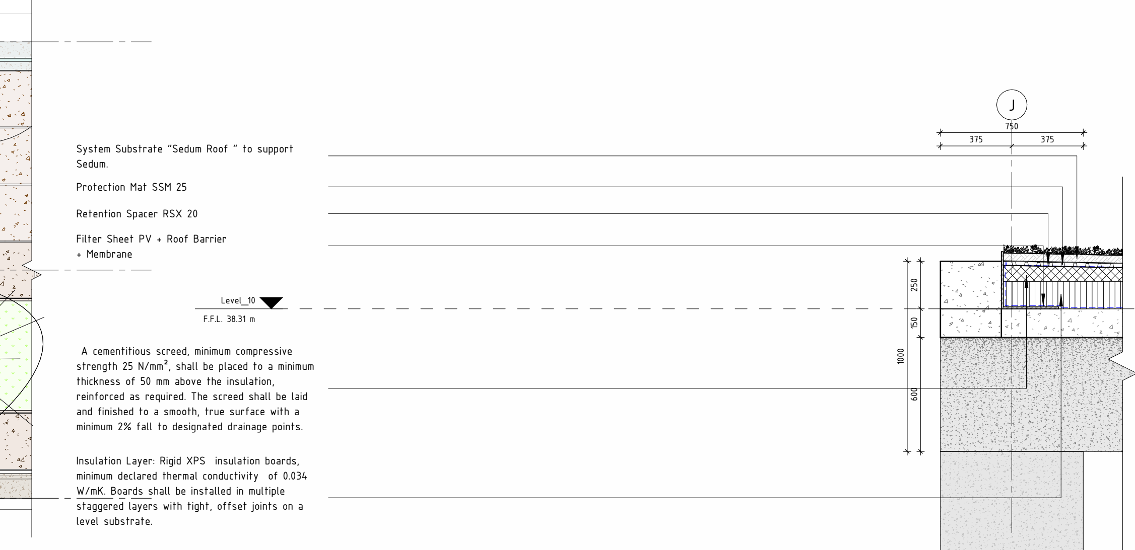
6 TYPICAL FACADE - DETAIL @ CANOPY EDGE 1:20
